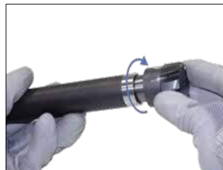
Hand-tighten the exchangeable head clockwise in the exchangeable head mount. Then clamp the exchangeable head mount along with the tool in the machine mount.
