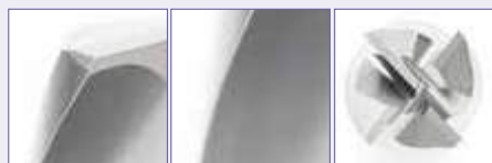
Dual cutting edge protection with edge protection chamfer and robust face-cutter Defined cutting edge honing increases the service life and process safety Radius-shaped gashing for improved chip removal
