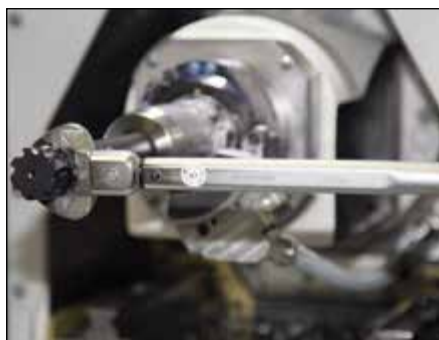
Tighten the exchangeable head using the torque wrench and the appropriate open-end snap-in spanner with the indicated tightening torque (see Table 'Exchangeable head tightening torque').
