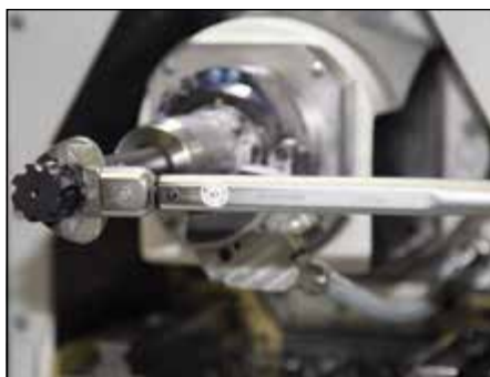
Place the torque wrench as horizontal as possible on the exchangeable head and ensure the wrench surface is not tilted.
