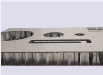
Alu honeycomb with GFRP cover
