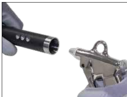
Clean the taper, thread and flat surface of the exchangeable head mount using compressed air and a cloth.
