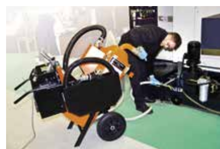
Returns the cleaned emulsion into the cooling lubricant container
