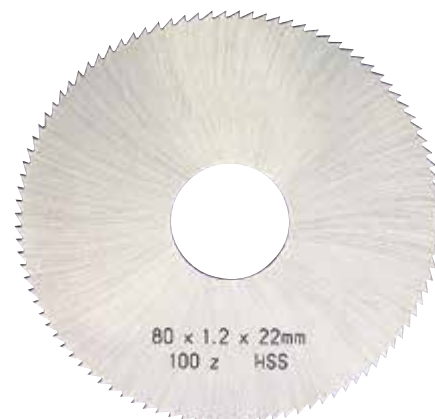
Fine-toothed, Form A, double helical tooth, DIN 1840 (rake angle 5°)
