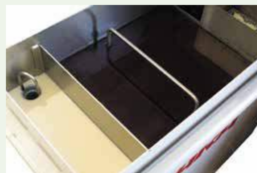
The oil collects on the surface of the resting basin (middle chamber).
