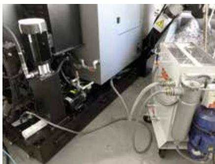
Control unit with pre-filter to protect the pump
