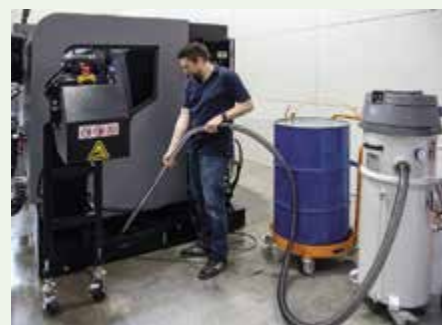
Bypass process extracts emulsion directly into the disposal container
