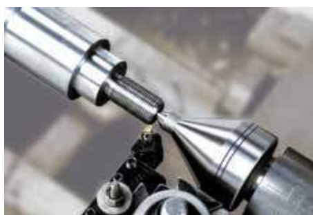
The extended running point guarantees the required clearance angle for turning parts with small diameters.
