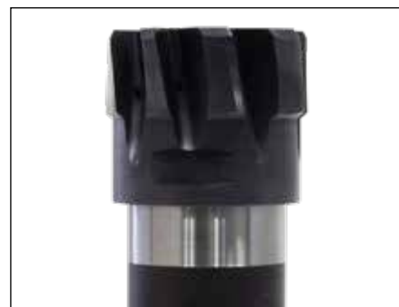
Result: the gap between the exchangeable head and exchangeable head holder is closed and the connection is force-fitting and positive-fitting. The exchangeable head is now ready for use.
