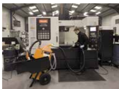
Vacuuming up dirty emulsion, chips and grinding sludge
