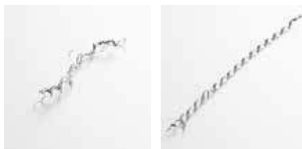
Chips from a conventional tap Chips from the CC-SFT
