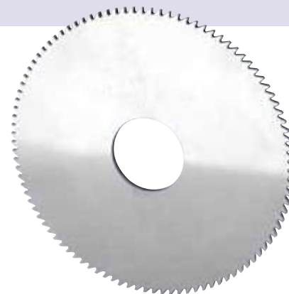
Fine-toothed, Form A, double helical tooth, DIN 1840 (rake angle 5°)
