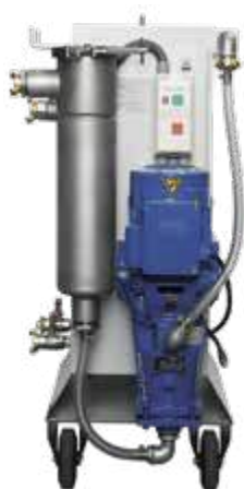
Control unit with pre-filter to protect the pump
