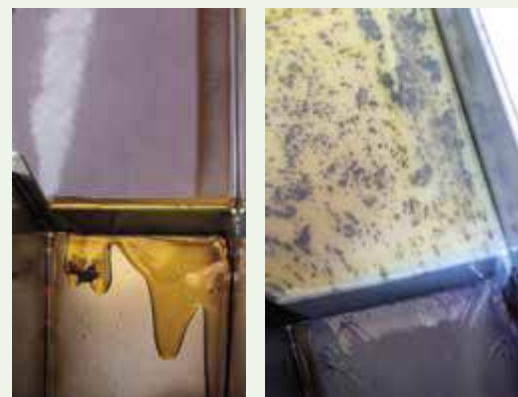
Changing the water level allows the collected oil to be drained off into the collection tank via a rounded edge.
