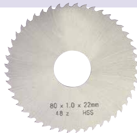
Coarse-toothed, Form B, curved tooth, DIN 1840 (rake angle 15°)
