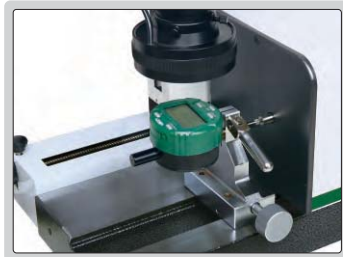
check digital indicators (detect digits on screen)
