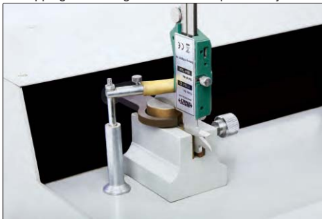
lapping measuring surfaces of caliper lower jaws
