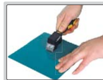
step 1: make grid cutting on surface
