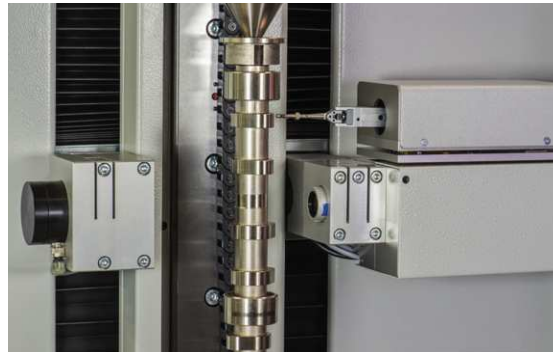
Tactile measuring unit with y-measuring axis 60 mm
