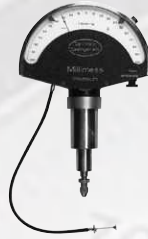
Millimess Dial Comparator - Built in 1937. The first indicating unit for reliably recording dimensional differences down to 1/1000 mm
