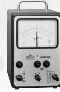
Millitron - Built in 1964. It is a compact length measuring instrument that was given the nickname "The Miner's Lamp"
