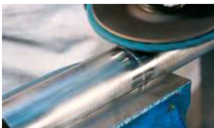
Sanding fine welding seams and removing thermal discolouration
