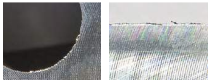
Before machining - Distinct burrs on the edge. Milling grooves on the surface.
