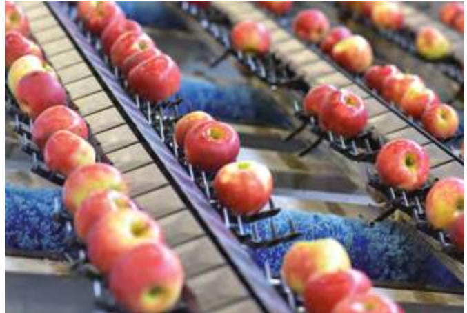
MultiZack® brushes are suitable for cleaning, transporting and polishing fruit or vegetables.
