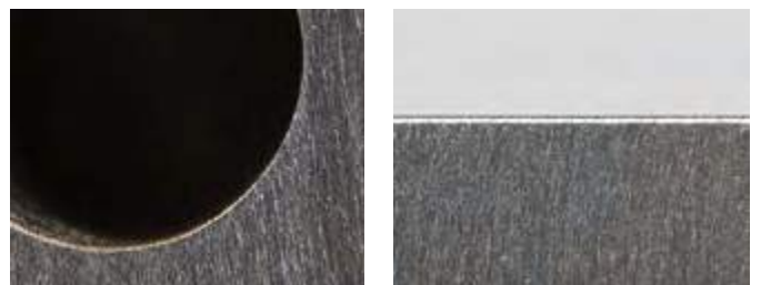
After machining - Burrs have been reliably removed and the edges rounded. The surface has a uniform, brushed appearance.
